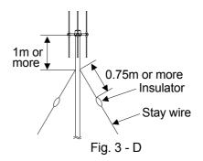
When an H type Adcock antenna is installed on board a small fishing boat 15m or smaller, please refer to the following figure.
