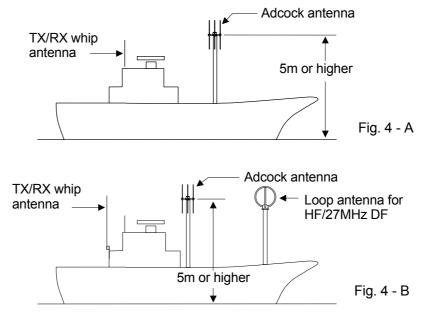
When a H type Adcock antenna is installed on board a fishing boat 20 ~ 30 m long or more, please refer to the following figure.
